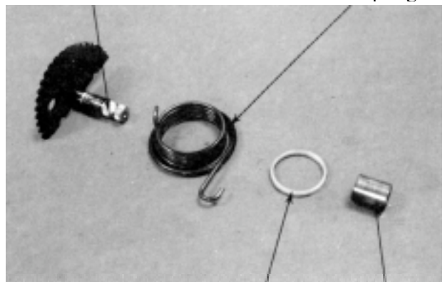
Plastic Bushing Spindle Bushing Friction Spring
