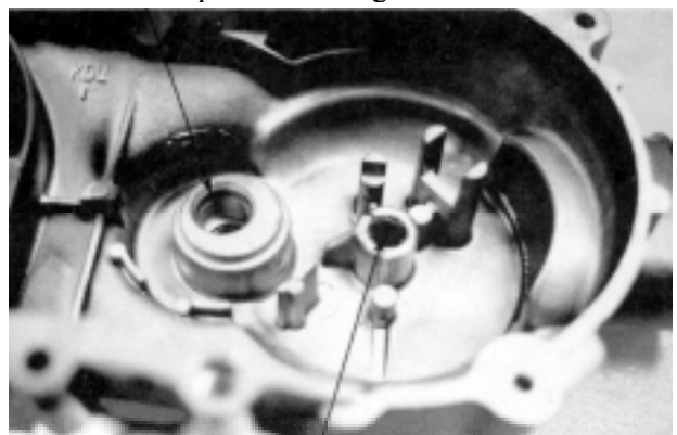
Starter Driven Gear Shaft Forcing
